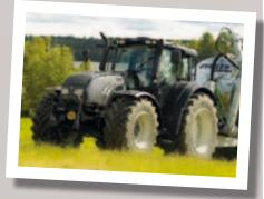
Valtra 202 featured the modern CVT transmission called Direct, which is a combination of mechanical and hydrostatic drive.
