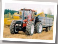
The Valmet H800 featured a fully hydrostatic transmission with no fixed mechanical transmission at all.
