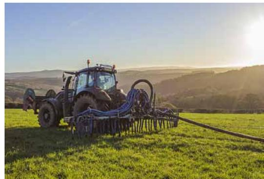
Umbilical slurry spreading will keep the T214D busy for many a day as one of its major tasks within the operations at B & B.
