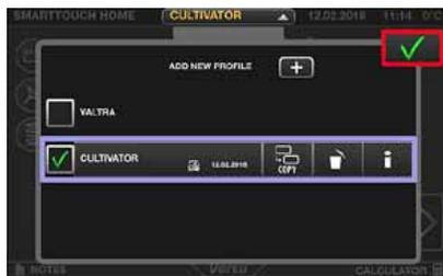
**1** Open the Profile menu from the top of the screen. To begin with you can select factory default settings or an existing profile as the basis for a new profile. For example, if you have already saved plough settings, they could serve as the basis for new cultivator settings. Name the new profile immediately so that you don't accidentally save on top of the old setting. You can save an unlimited number of profiles in the settings.
