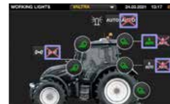
Configure the work lights easily with the 9" touchscreen. Premium and Premium+ work lights also include settable cornering lights, which are controlled by wheel angle sensor in the front axle.
