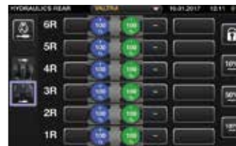
You can assign any control to operate any hydraulic function, including front and rear hydraulic valves, front and rear linkages and the front loader.
